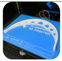
1. Immediately after modeling, there is an auxiliary floor to prevent wall collapse, so remove this auxiliary floor.
