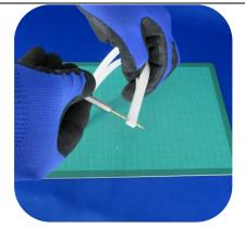
4. Insert a drill of about 3 mm into the holes on both ends, turn it by hand and go to the back to remove unnecessary items.
